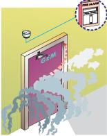
The Electromagnetic door holder automatically releases the armature plate allowing the door to close and preventing the fire and smoke from spreading.
